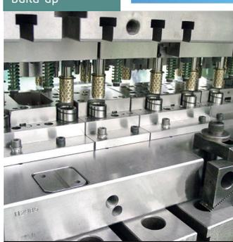
material utilization and the complexity of the die. Tools can be designed to produce individual loose laminations and/or designed to stack laminations in the tool through mechanical interlocking or gluing.
